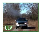
The ULVs break the chemical down into small droplets of 15 microns (a human hair is 100 microns in diameter) allowing the chemical to be carried by the air currents to reach the target area. The ULV sprayers are the units approved by the world health organization and used by most other companies. All our trucks are equipped with ulvs even though use of them is very limited because they are not near as effective as TUG units
